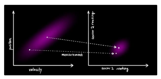
Notice that the units and scale of the reading might not be the same as the units and scale of the state we're keeping track of. You might be able to guess where this is going: We'll model the sensors with a matrix,  $\mathbf{H}_k$ .
