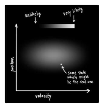
The Kalman filter assumes that both variables (postion and velocity, in our case) are random and *Gaussian distributed*. Each variable has a **mean** value  $\mu$ , which is the center of the random distribution (and its most likely state), and a **variance**  $\sigma^2$ , which is the uncertainty:
